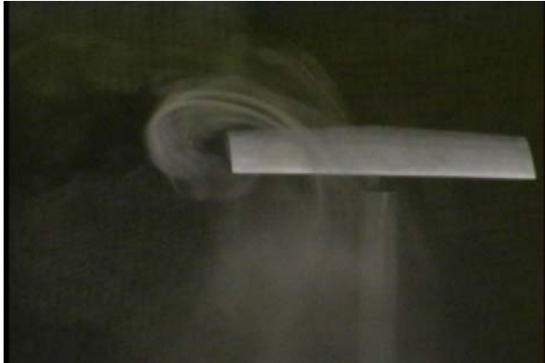
Figure 1. Flow-visualization of the tip-vortex for the MAV without a winglet.
