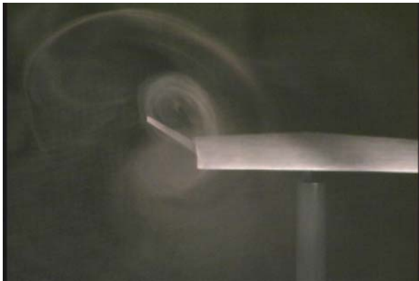
Figure 2. Flow-visualization of the tip-vortex for the MAV with a winglet.
